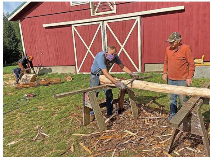
Stephen Bear from Texas strips bark off a cedar log to make fence posts while camp ranger Rocky Schlager looks on. In the background, Darryl Ueek from Alaska sharpens his chainsaw.
