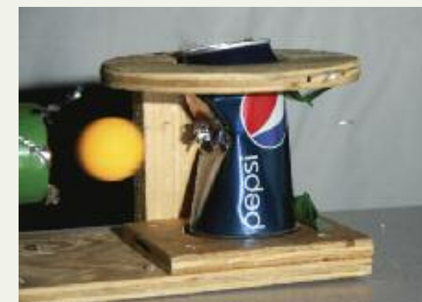
Notice that the can is bent even though the ball has not come close. Evidence of the high-speed shock wave is given by the pieces of silver polymer membrane flying by the can. It is this shock wave that sounds like an explosion and triggers the flash.
