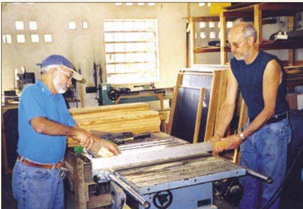
Sam Pellecer, left, and Henry Geppert cut frames for window screens.
