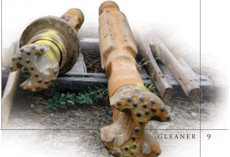
These heavy bits are lifted and dropped about 60 times a minute to drill a well.
