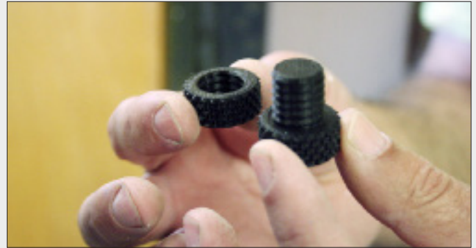
These parts were created with PAA's new 3-D printer, the MakerBot. Art students get a rare opportunity to create three-dimensional objects with 3-D design software Rhino and then print their designs on the MakerBot.
