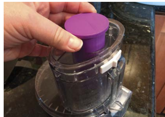
The teacher printed a Cuisinart food processor plunger to replace a missing one.
