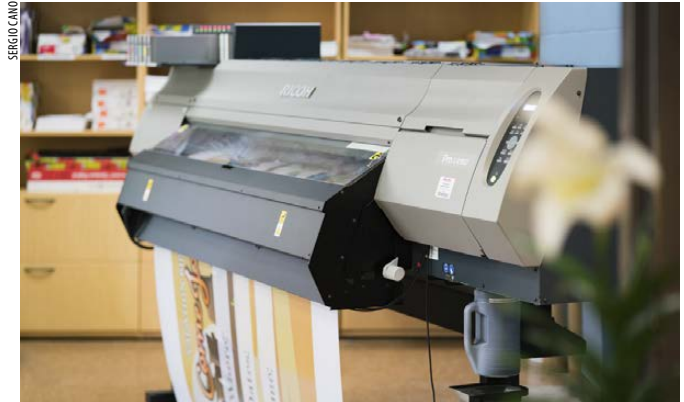
The 63-inch banner printer can print canvas or vinyl banners, posters, and window-clings.
