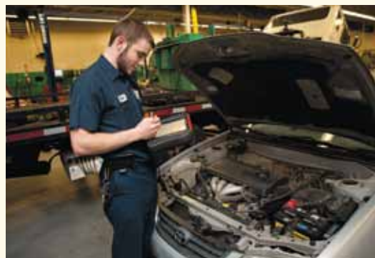
Students receive vehicle inspection training using diagnostic scanners in the Technology Department's on-campus auto shop.
