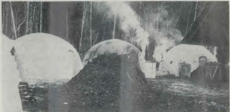
To help pay for the clearing of the land, trees cut down are brought to this site where they are made into charcoal and then sold or used to help "sweeten" the soil for planting. The excessive acidity of the soil, due to tannic acid, must be reduced for better growing.
