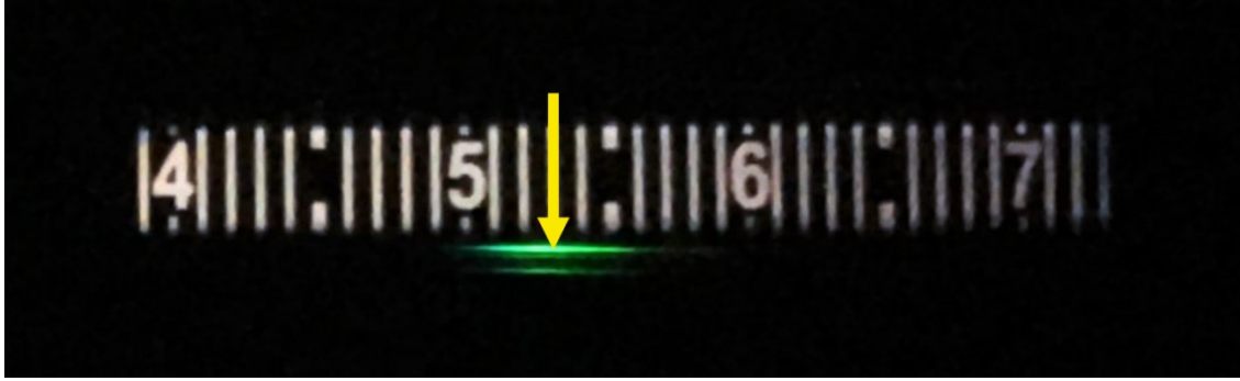
Fig. 11: Image of spectrum produced by a green LED with central wavelength indicated.
