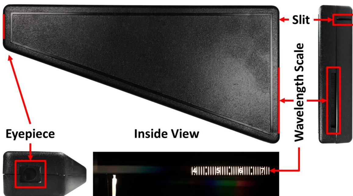
Fig. 4: Handheld spectroscope with eyepiece, vertical slit, and wavelength scale.
