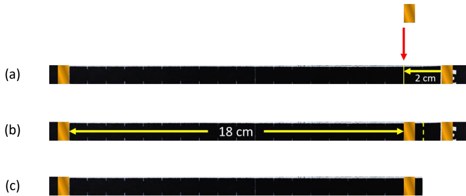
Fig. 5: (a) Apply another piece of conductive tape 2 cm over so that the new length between conductive tape strips is 18 cm. (b, c) Cut the paper between the new and old tape strips (dashed line) to make a shorter paper strip with an 18 cm separation between the pieces of conductive tape.
